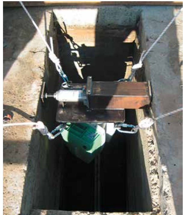
Fig 4: Inverted scanner with engineered bracket
