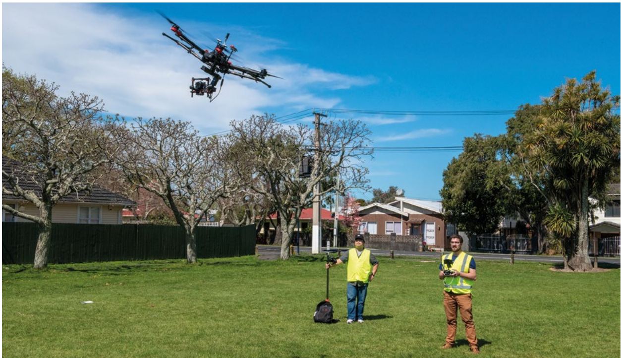
Jonathan demonstrates the versatility of a multi-rotor, together with the stability of a camera with a gimbal attachment.
