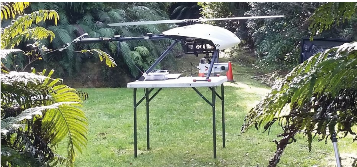
Rodney's impressive single rotor ORC from Altus can take a large payload easily, such as the LiDAR unit, and has a flight time of up to 45 minutes on a single battery.
