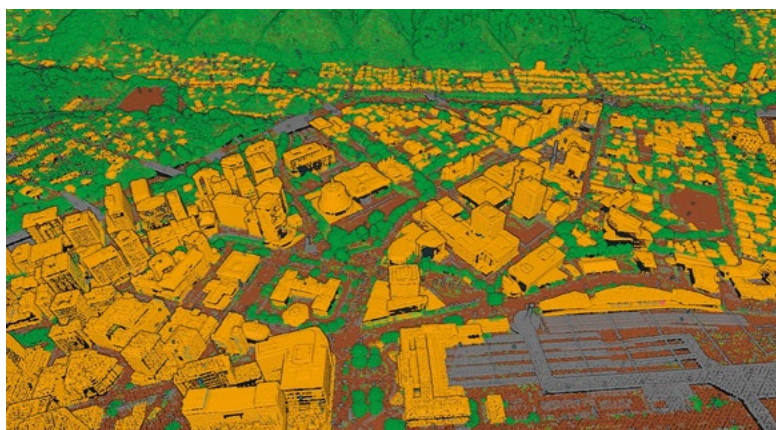
Wellington City 2019-2020 Point Cloud. A point cloud is all the data points captured before they are processed to produce the DEM or DSM. Point clouds are often viewed in 3D as a cloud of points, hence the name. The data points are classified into feature types, including things like bare ground, water, vegetation groups and buildings. These further enable users to apply the data to many purposes.
