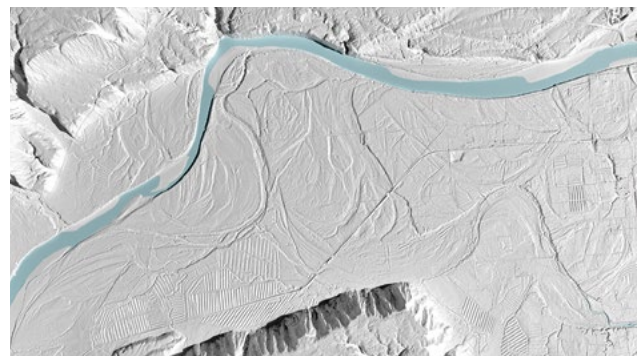
A digital elevation model from the recent Westport area survey, part of the West Coast Regional Council's project to provide full regional coverage. The data revealed the detail of geomorphological features including past river channels and land altered by farming.
