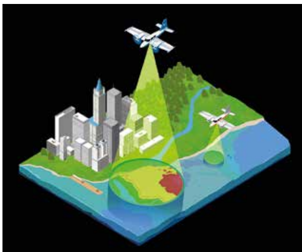
Diagram of increased LiDAR being captured by higher flying vessels (Daniel Kruimel AAM/Woolpert).
