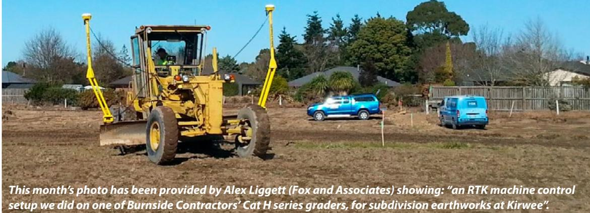
*This month's photo has been provided by Alex Liggett (Fox and Associates) showing: "an RTK machine control setup we did on one of Burnside Contractors' Cat H series graders, for subdivision earthworks at Kirwee".*
