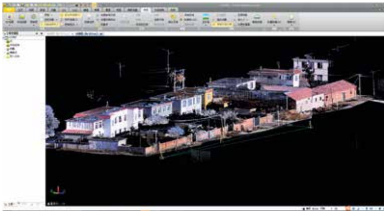
Technicians blended point clouds and images to produce 3D visualisations of Changchun buildings. The image includes locations of SX10 setup stations.
