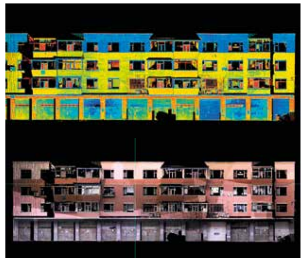
Examples of raw data (top) and finished elevation in Trimble Business Centre. Results could be exported to standard CAD software and formats.
