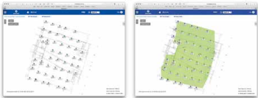
Figure 11 – Final result of the displacement of the columns and iso-lines representation for quick understanding
