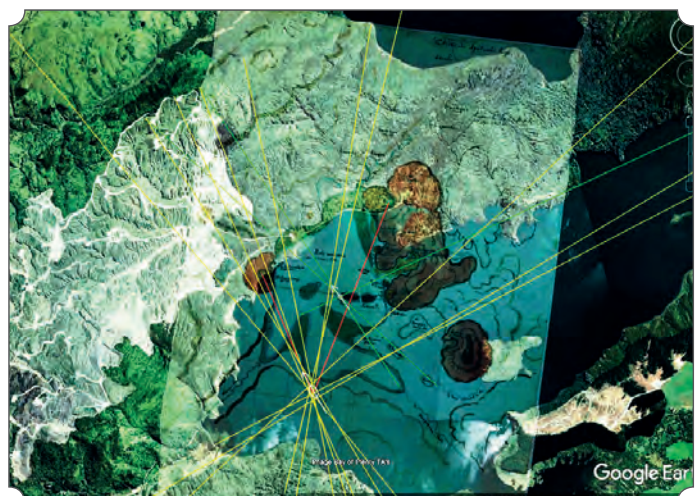
Figure 8: Close-up of the Iteration Five resection, 10 bearings (yellow) on Station 21 and three bearings (green) on Station 22. The two red bearings are to the Tarata and Otukapuarangi Springs, from Station 21 (Bunn April 2, 2018).
