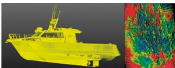
Fig 8: University of Otago survey vessel and seabed imagery collected with the R2 Sonic 2026 multibeam (Source: School of Surveying & E. Tidey).
