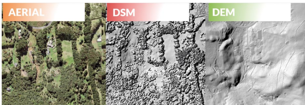
Figure 5 – Difference between DEM and DSM surfaces with aerial imager for visual reference.
