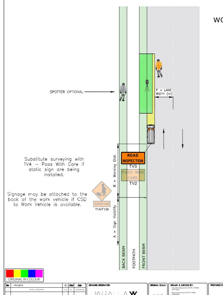
**OPERATION 9 - LR/LV AND LOW VOLUME ROADS** WORKING WHERE THERE IS NO EDGE LINE OR INFERRED EDGE LINE **TRIPOD STRADDLING THE KERB & CHANNEL OVERTAKING VEHICLES NOT CROSSING CENTRELINE** OR ENTERING THE FLUSH MEDIAN (ENTERING THE LIVE LANE)
