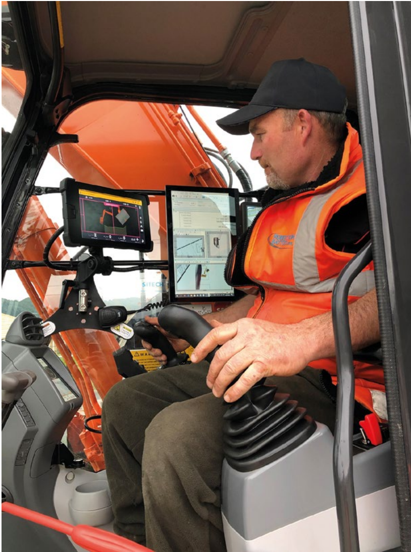
Figure 2: Conrad Robertson from Robertson Battock Civil uses both grade control and avoidance zone GNSS technology.
