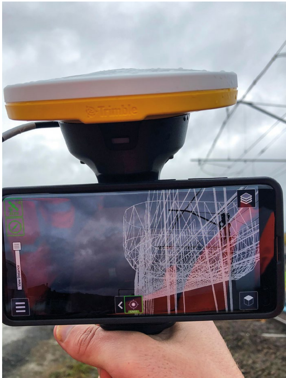
Figure 3: Data validation using Trimble SiteVision.
