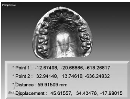
Figure 7: Slope distance measurement on dental cast surface 3D model.
