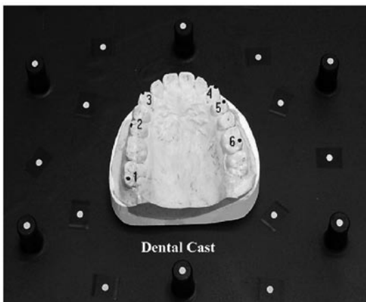
Figure 3: The dental cast and the scanning configuration.
