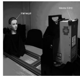
Figure 8: The mannequin and the scanner during the scanning. Note that the holding device can rotate the scanner along its vertical axis.
