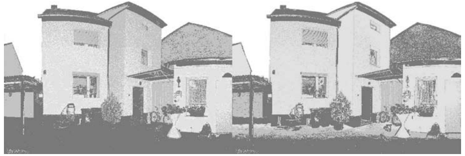
Figure 8: Segmentation of the calibrated point cloud [left] and the calibrated and corrected dataset [right].
